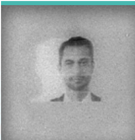
Hidden ghost image invisible image under the colour-changing print, verifiable by IR cameras
